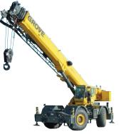
The RT700E has a quick-reeve boom nose and swingaway alignment device to help operators set up smoothly.
