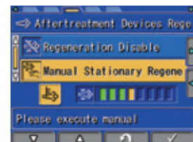
Aftertreatment device regeneration screen
